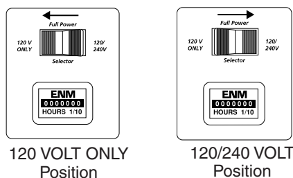
Figure 3 - Full Power Selector Switch
